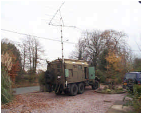
Picture right : The truck roof showing left to right the aerial storage lockers, The new VHF 2m collinear on top of the log-periodic (in green bags) and the flexible exhaust extension for the generator.
