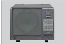
SP-20 EXTERNAL SPEAKER 4 audio filters; headphone jack; can connect to 2 transceivers. Input impedance: 8 \Omega . Max. input power: 5W
