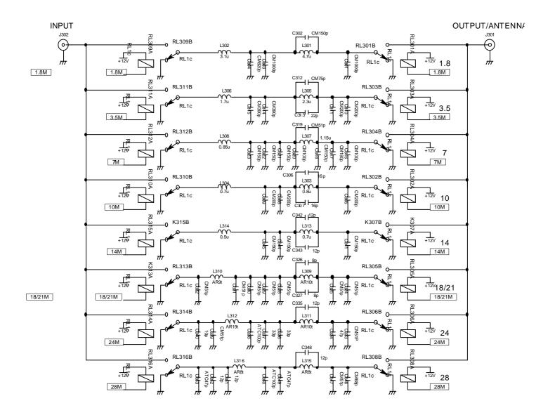
The filter section consists of eight(8) band-division low pass filters to be selected by IN/OUT relays of the respective bands.
