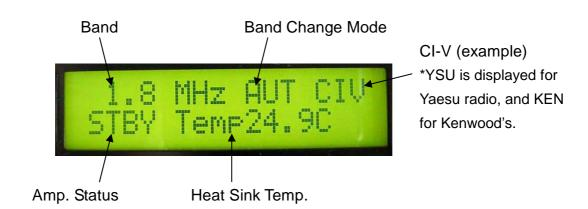
**LCD Panel** Displays modes of operation and protection circuit.
