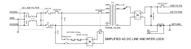
AC mains are indirectly turned on by the Main Relay. In series to this relay, there are connected thermal switches for PA heat sink (100 ) and power transformer (130 ) that work independently from other electronic protection circuits. Threshold values are set much higher than other protections, and they do not turn on in the normal operating conditions.
