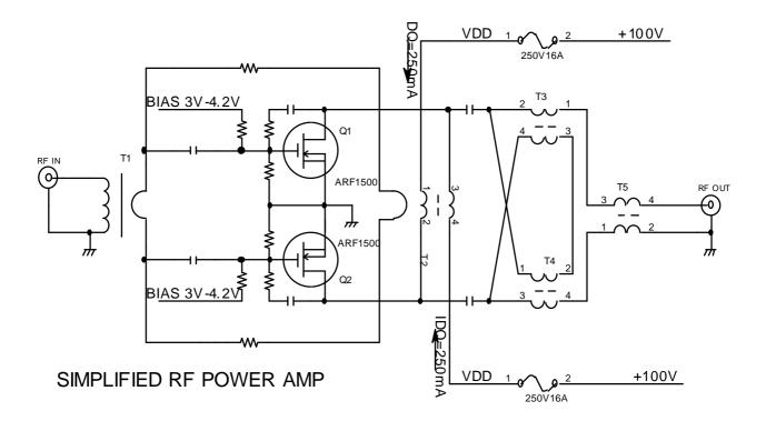
PA consists of a pair of Microsemi ARF1500, in class AB push-pull configuration.
