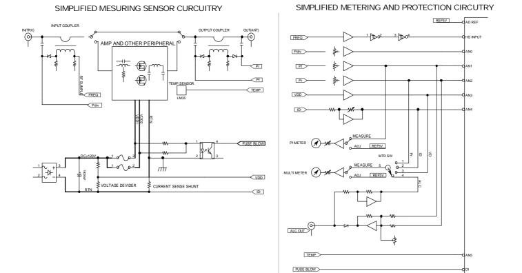
All the analog sensors of HL-2.5KFX are scaled to be 0 to 5V range and are numerically controlled by ten bit AD converter of MPU (PIC16F472).
