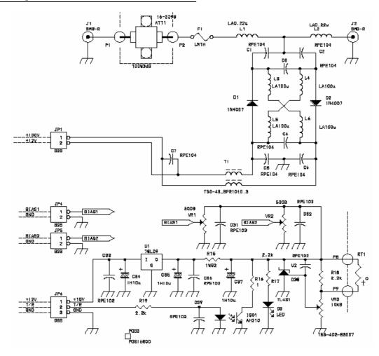
To set the input (drive) power level of the amplifier to be 100W, 3dB power attenuator is built in the input side.
