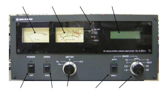
**POWER** Main power switch to turn AC power on and off.
