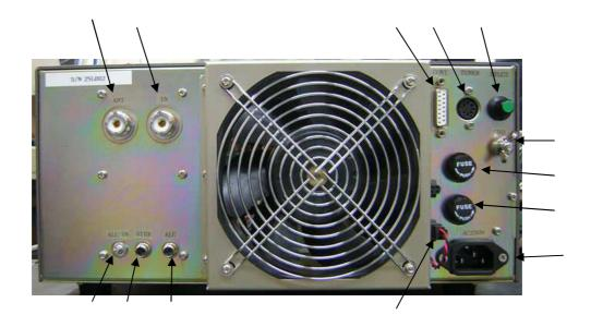
**ANT A** RF Output Connector. Connect the coax cable to the antenna.
