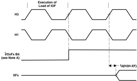
NOTE A:  $\overline{1}$ /OxFx represents either bit 1 or bit 5 of the IOF register.
