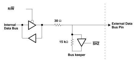
Figure 9. Bus Keeper Circuit
