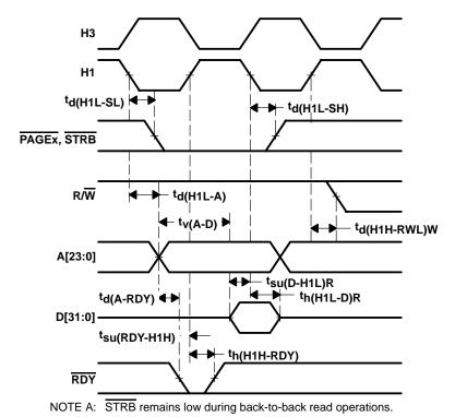
Figure 20. Timing for Memory ( $\overline{STRB} = 0$  and  $\overline{PAGEx} = 0$ ) Read
