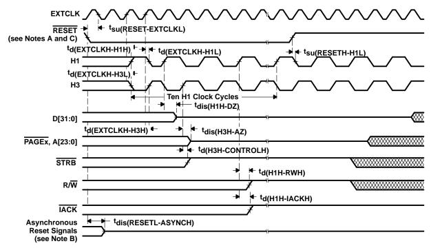
NOTES: A. Clock circuit is configured in 'C31-compatible divide-by-2 mode. If configured for x1 mode, EXTCLK directly drives H3.
