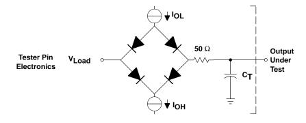
Where:  $I_{OL}$  = 4 mA (all outputs) for DC levels test.
