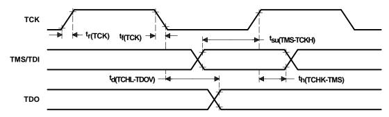
Figure 40. IEEE-1149.1 Test Access Port Timings
