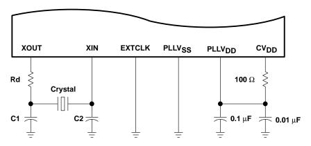
Figure 5. Self-Oscillation Mode
