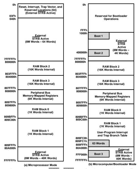
NOTE A: STRB is active over all external memory ranges. PAGE0 to PAGE3 are configured as external bus strobes. These are simple decoded strobes that have no configuration registers and are active only during external bus activity over the following ranges:
