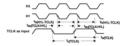
Figure 37. Timer Pin Timing, Input
