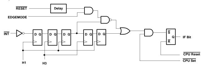
Figure 7. EDGEMODE and Interrupt Flag Circuit
