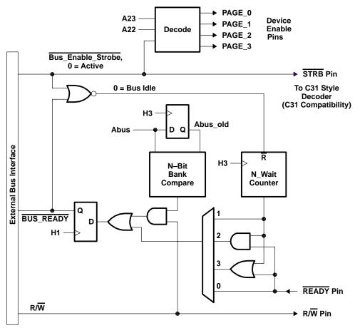
Figure 8. Internal Ready Logic, Simplified Diagram
