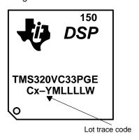
Figure 13. PGE Package (Top View)
