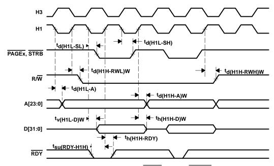
Figure 21. Timing for Memory ( $\overline{STRB} = 0$  and  $\overline{PAGEx} = 0$ ) Write
