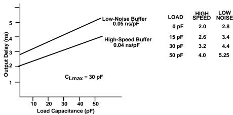
Figure 19. Output Load Characteristics, Buffer Only
