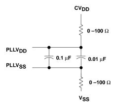
Figure 6. PLL Isolation Circuit Diagram
