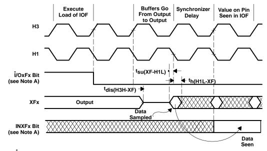
NOTE A: I/OxFx represents either bit 1 or bit 5 of the IOF register, and INXFx represents either bit 3 or bit 7 of the IOF register.
