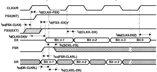
Figure 31. Fixed Data-Rate Mode Timing
