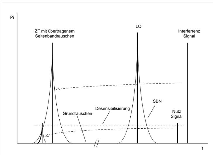
Figure 2: Dynamic range reduction due to reciprocal mixing
