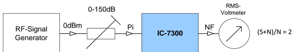
**Fig. 1: Measurement setup to determine sensitivity (MDS, minimum discernible signal)**
