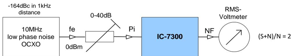
Figure 3: Test setup for RMDR and SBN measurement
