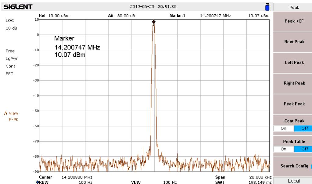
Figure 12: Maximum HF output power in the 20m band
