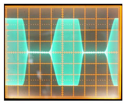
Figure 21: Keying envelope at 48 wpm, 1:3:1 weight, rise time 6 ms.
