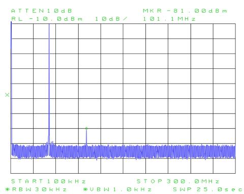
16. AM sidebands and THD with single-tone modulation. As in Test 15 above, the spectrum analyser is connected to ANT1 via a 50 dB high-power attenuator. RF PWR is adjusted for 50W resting carrier. A 1 kHz test tone is applied from the HP 8935 test set to A ACC1 Pin 4 (MOD IN). AM sidebands are measured using the HP 85672A spurious response utility.
