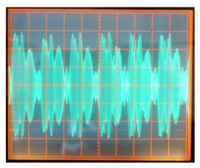
10. ALC Compression Check. In this test, a 2-tone test signal is applied to A ACC1 Pin 4 (MOD IN) from an HP/Agilent 8935 test set. The terminated oscilloscope is connected to ANT1 via a 50 dB high-power attenuator.
