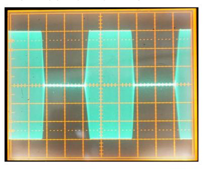
19. **Comments on receiver test results:** The **NPR** test data (Test 2) show an improvement of several dB over the IC-7700 and IC-7800, mostly attributable to the IC-7851's 30+ dB RMDR improvement over earlier designs. NPR values ≥ 90 dB approach the measurement limits of the instrumentation. It will be noted that with the 1.2 kHz roofing filter selected, NPR is a few dB lower than with the other roofing filters. This is suggestive of PIM in the 1.2 kHz filter under high noise loading.
