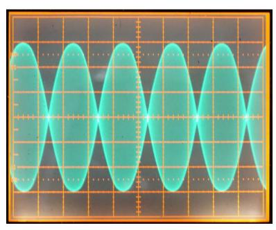
ALC Overshoot Test with White Noise. In this test, white noise is applied applied to A ACC1 Pin 4 (MOD IN) from an HP 8935 test set. The terminated oscilloscope is connected to ANT1 via a 50 dB high-power attenuator.
