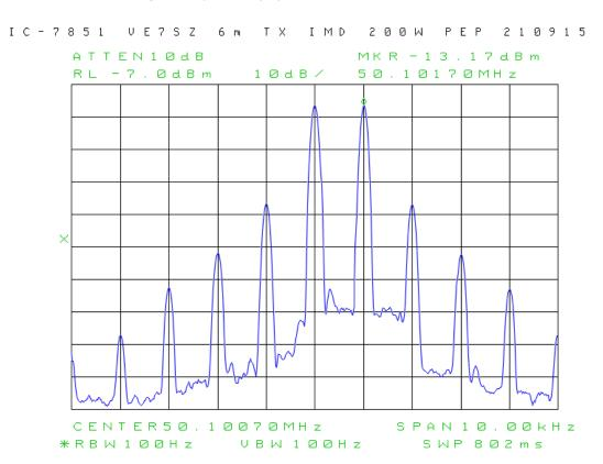
Figure 10: Spectral display of 2-tone IMD at 28.3 MHz, 200W PEP.
