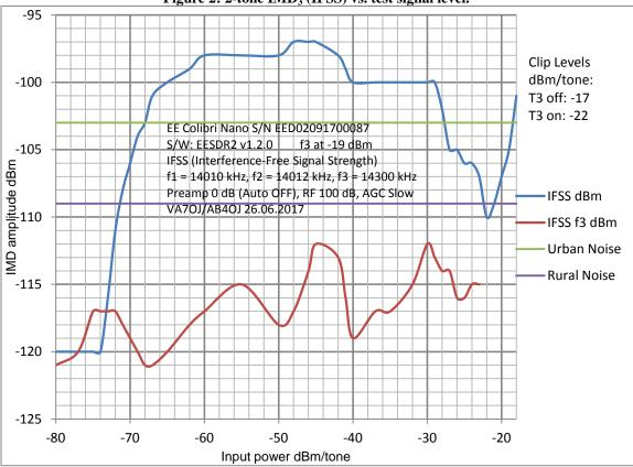
Figure 2: 2-tone IMD<sub>3</sub> (IFSS) vs. test signal level.
