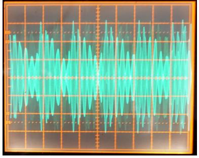
15. ALC Compression Check. In this test, a 2-tone test signal is applied to the MIC jack from an audio generator. An oscilloscope is connected to ANT3 via a 45 dB high-power attenuator.
