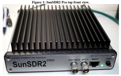
*Introduction:* This test report presents results of an RF lab test suite performed on a SunSDR2 Pro direct-sampling/DUC SDR transceiver kindly loaned by Yuri Sushkin N3QQ.
