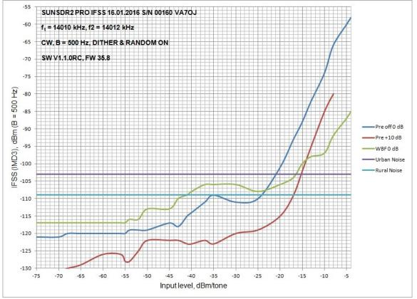
Figure 23: IFSS (2-tone IMD<sub>3</sub>) vs. test signal level.
