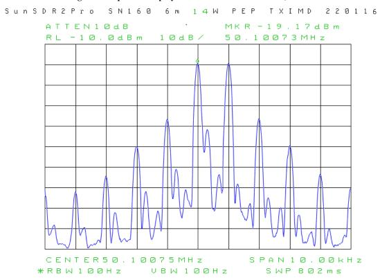
Figure 26: Spectral display of 2-tone IMD at 50.1 MHz, 14W PEP.
