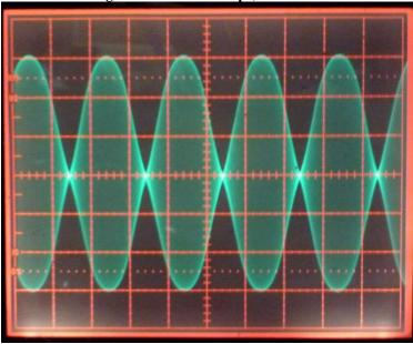
*15a: Subjective TX audio test:* In this test, a headset is plugged into the microphone and headphone jacks and a transmitted SSB signal is monitored with MON active.
