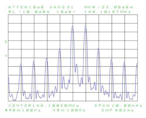
17: Transmitter harmonics & spectral purity. Once again, the spectrum analyser is connected to the ANT3 (HF) or ANT1 (2m) via a 55 dB high-power attenuator. Tone is set at 100%. The spectrum analyser's harmonic capture utility is started.
