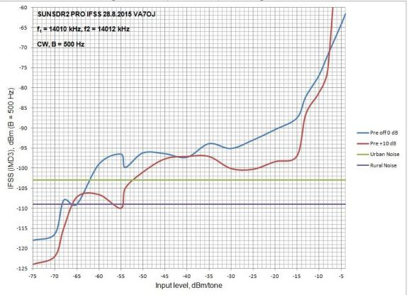
Figure 5: IFSS (2-tone IMD<sub>3</sub>) vs. test signal level.
