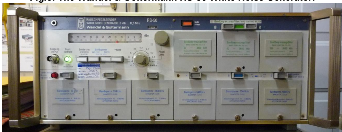
Fig.6: The Wandel & Goltermann RS-50 White Noise Generator.
