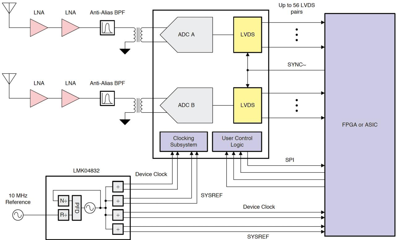
3. Here, a direct-sampling software-defined radio is using TI's 12-bit, 6.4-Gsample/s ADC12DL3200 with LVDS.
