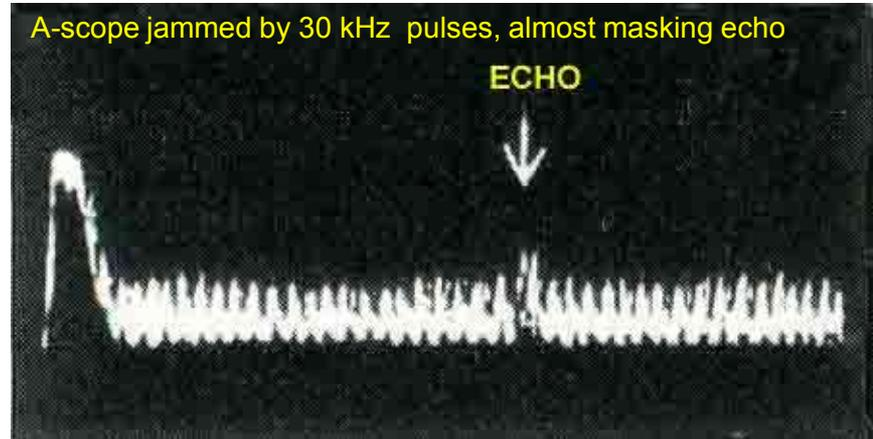
A-scope jammed by high-power noise-modulated signal
