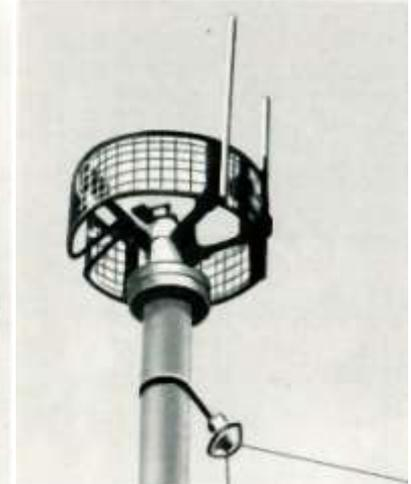
Newer U-boat mounted *Bali* circular dipole (90-470 MHz).
