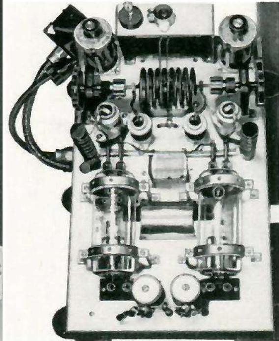
1 kW transmitter chassis
