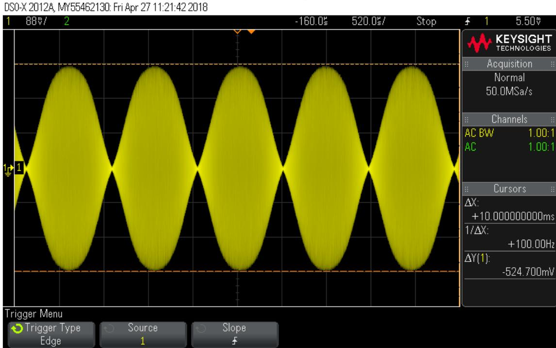
**21a: Subjective TX audio test:** In this test, a headset is plugged into the microphone and headphone jacks and a transmitted SSB signal is monitored with MON active.
