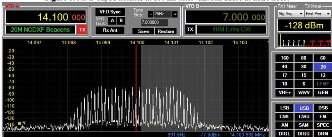
**7: AGC impulse response.** The purpose of this test is to determine the Anan-7000DLE's AGC response in the presence of fast-rising impulsive RF events. Pulse trains with short rise times are applied to the receiver input.
