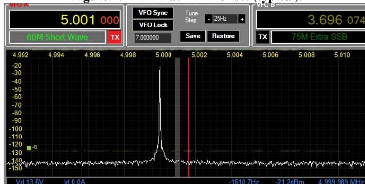
**3: Channel filter shape factor (-6/-60 dB).** This is the ratio of the -60 dB bandwidth to the -6 dB bandwidth, which is a figure of merit for the filter's adjacent-channel rejection. The lower the shape factor, the “tighter” the filter.
