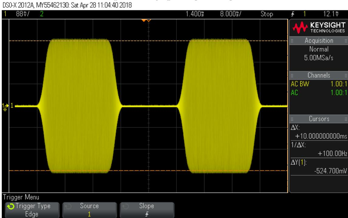
**28: CW QSK recovery test.** This test has been devised to measure the maximum speed at which the receiver can still be heard between code elements in QSK CW mode.
