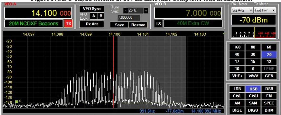
Figure 6: MNF on, 21 notches at 100 Hz intervals. RX audio at noise floor.
