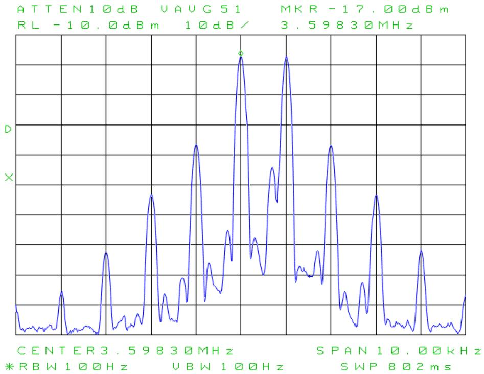
Figure 25: Spectral display of 2-tone IMD at 14.1 MHz, 20W PEP.
