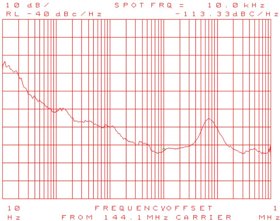
**20: Spectral display of CW keying sidebands.** The spectrum analyser is connected to ANT3 via a 55 dB high-power attenuator. The -10 dBm reference level equates to 100W. A series of dits is transmitted at 60 wpm.
