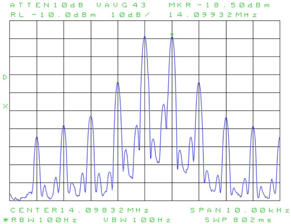
**Figure 12: Spectral display of 2-tone IMD at 50.1 MHz, 13.5W PEP.**
