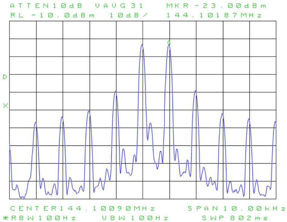
**17: Transmitter harmonics & spectral purity.** Once again, the spectrum analyser is connected to the ANT3 (HF) or ANT1 (2m) via a 55 dB high-power attenuator. Tone is set at 100%. The spectrum analyser's harmonic capture utility is started.
