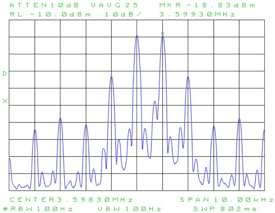
**Figure 11: Spectral display of 2-tone IMD at 14.1 MHz, 18W PEP.**
