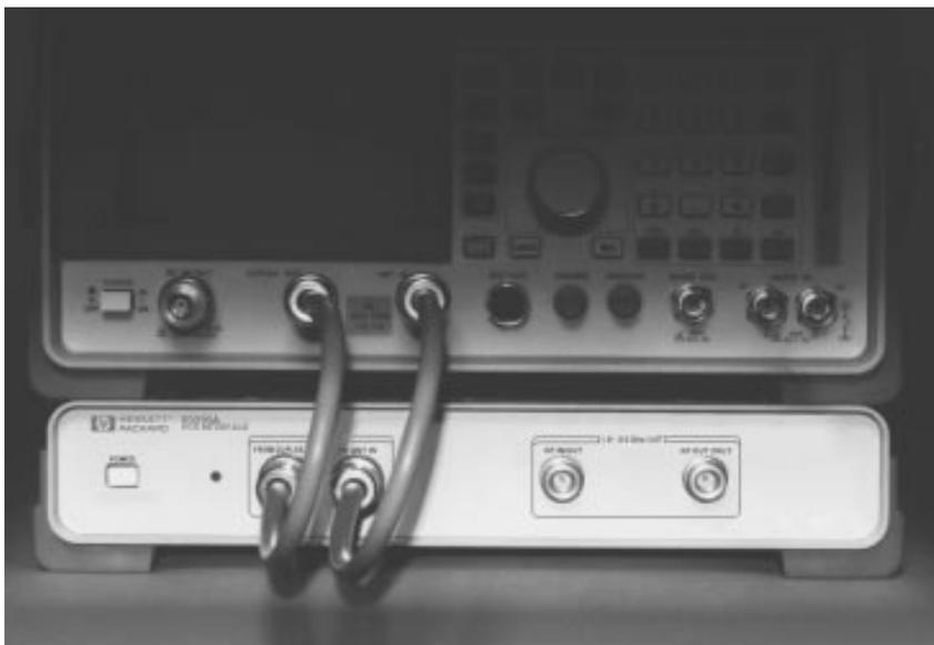
The HP 83236A is controlled via HP-IB for base station test. For manufacturing test, HP-IB commands written by the operator can be executed from an external controller, or from the IBASIC controller built into the HP 8921A. The HP 83224A IBASIC Developers Tool Kit is available for programmers who are new to IBASIC language programs for the HP 8921A. For more information on the Developers Tool Kit, refer to HP 83224A product overview, part number 5964-3897E.
